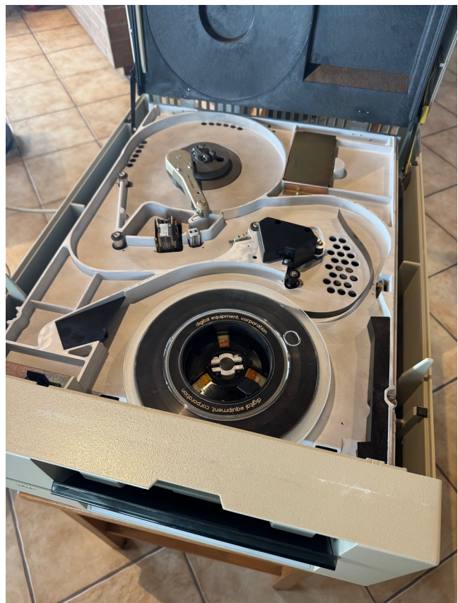
Internal tape chamber
