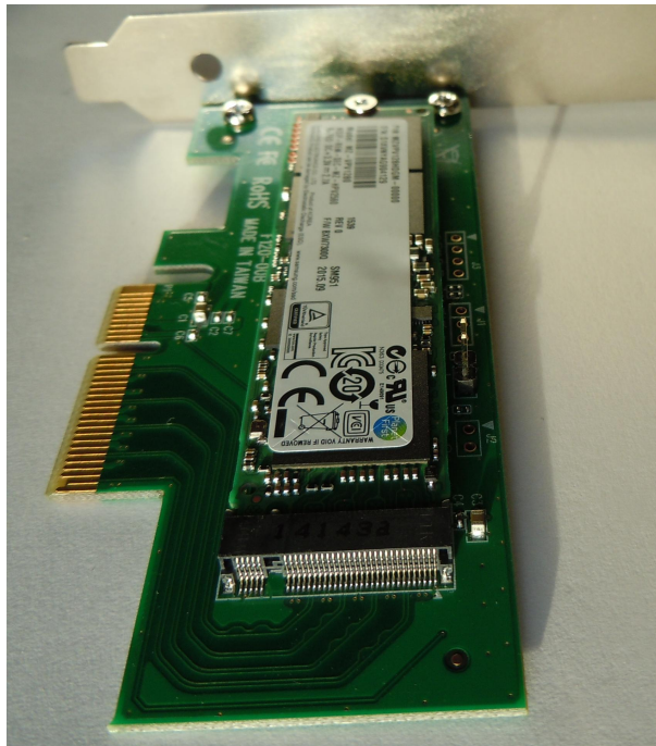
Figure 4: Samsung 951 (NVME) and a M.2 to PCIE slot adapter
